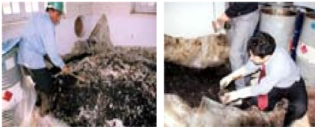
Fig. B.1: Mixing and sampling of petroleum sludge during bioremediation.
