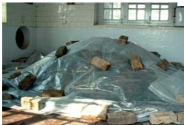
Fig. B.2: Sludge placed on plastic sheet and covered by plastic sheet
