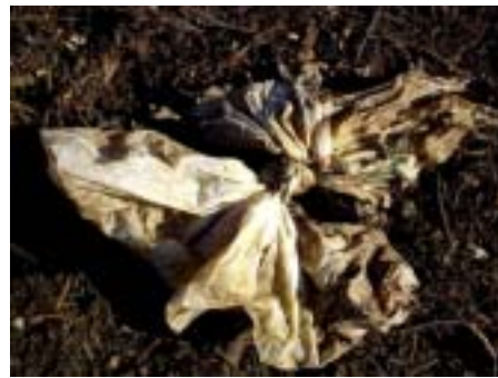
Picture 16. A knotted biodegradable bag after 1 week of composting
